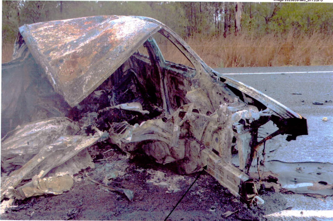
Picture showing the front left chassis rail relatively undamaged from impact
