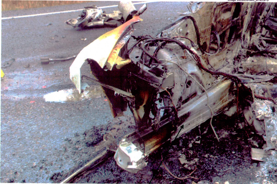
Picture showing the front right chassis rail relatively undamaged from impact
