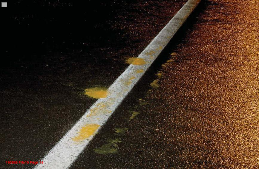
**Photograph No. 5:** Photograph of the short tyre mark on the fog line.
