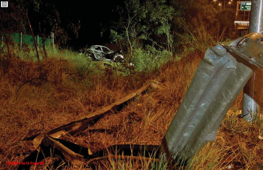
Photograph No. 8: View looking towards the vehicle in situ with the damaged section of w-beam in the foreground. The flattened grass around the w-beam is evidence of the passage of the vehicle through that area – the vehicle track mark.
