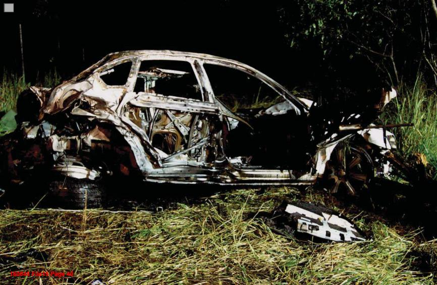
Photograph No. 16: View of the right (driver's) sid in its final rest position. This photo shows the deform rear end, including the rear wheel broken from the ax
