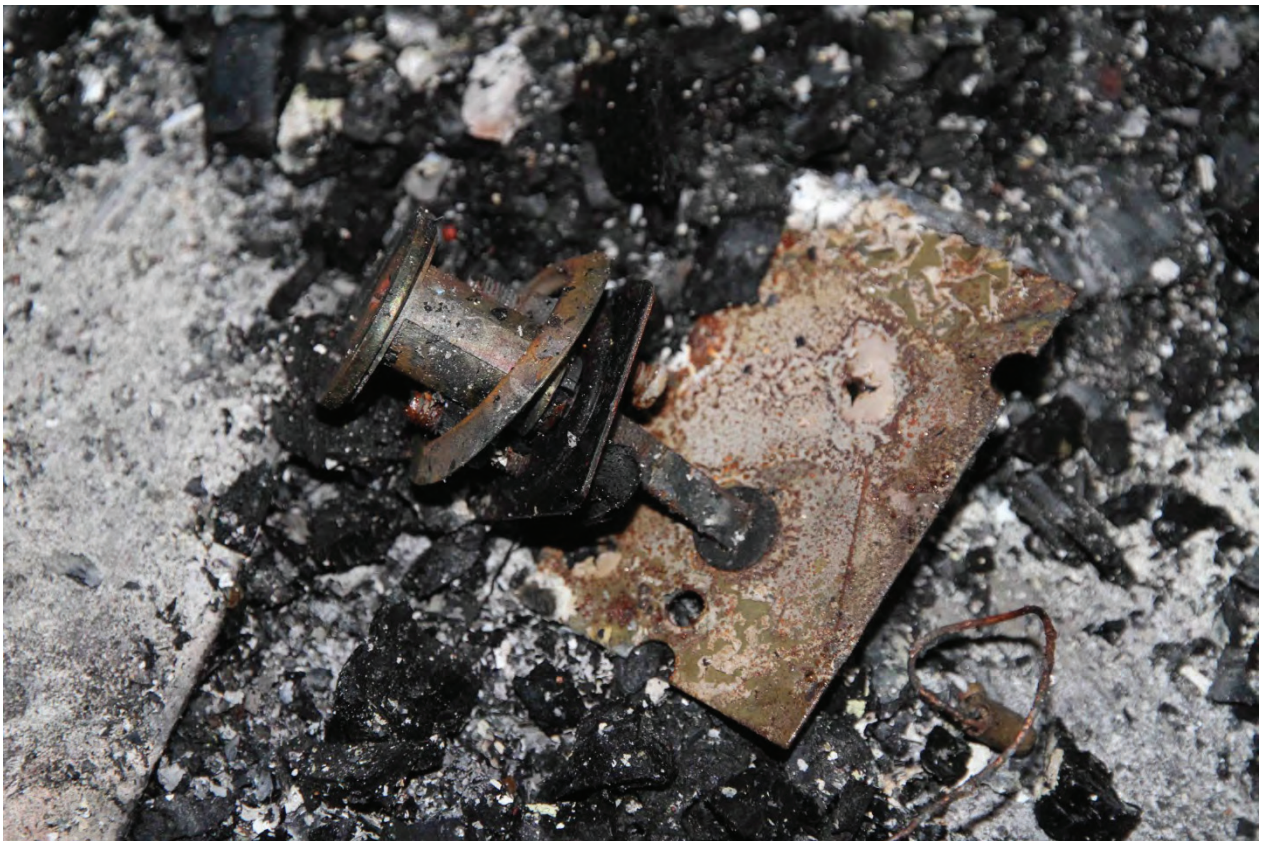
Figure 9. Showing the remains of the side door lock of unit 4.
